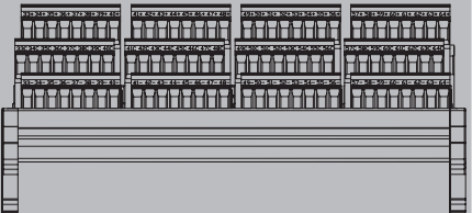
Field terminals view for ADV161 (Channels 33 to 64)
