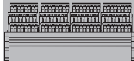
Field terminals view for ADV161 (Channels 33 to 64)
