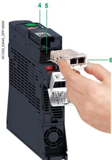
Example of installing a communication module 6
