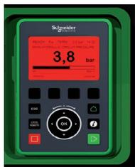
Detected fault: Red screen when there is a detected error
